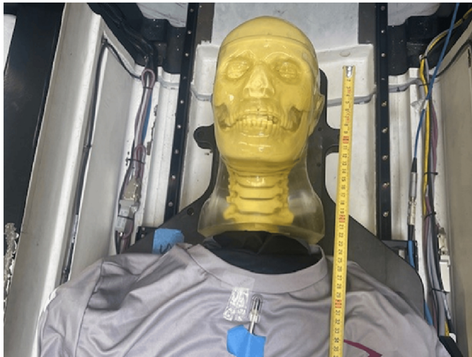
FIGURE 2: Measurement setup with the detector position
