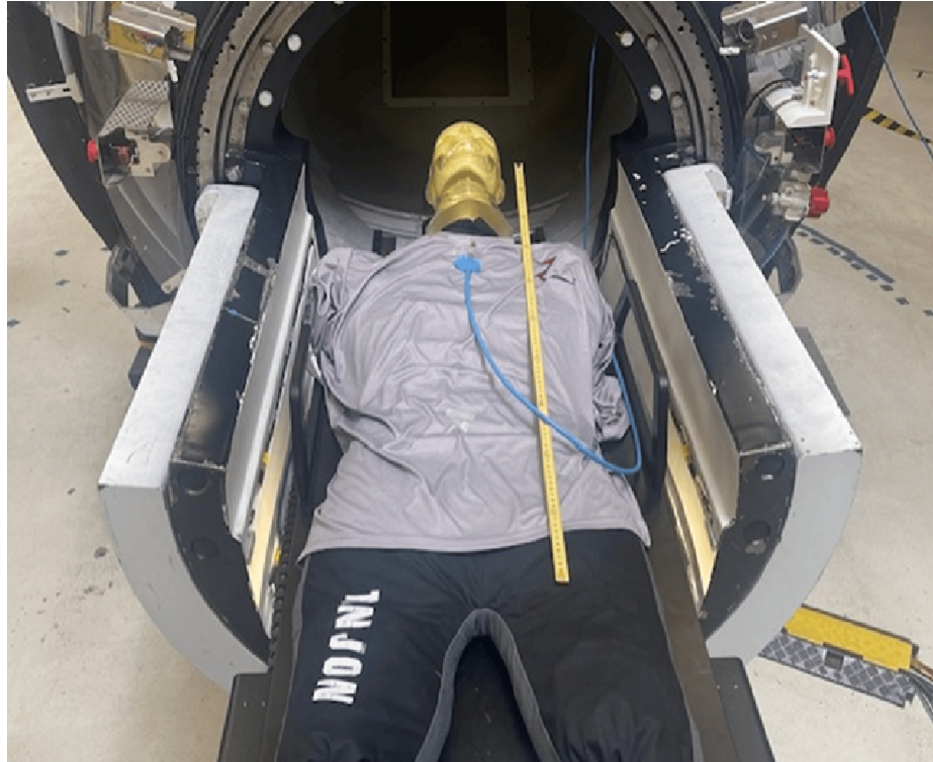
FIGURE 1: Phantom and test setup on the ZAP-X system
