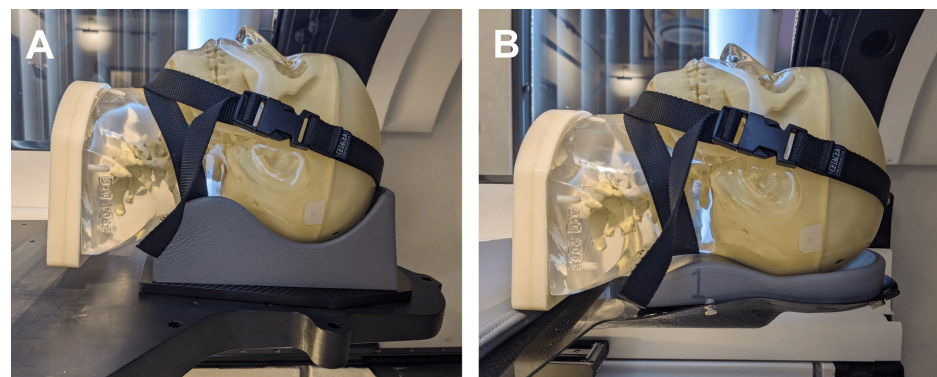
FIGURE 1: Setup of headrests with an anthropomorphic head phantom from the previous GRS (A) and updated GRS* (B) platform.
