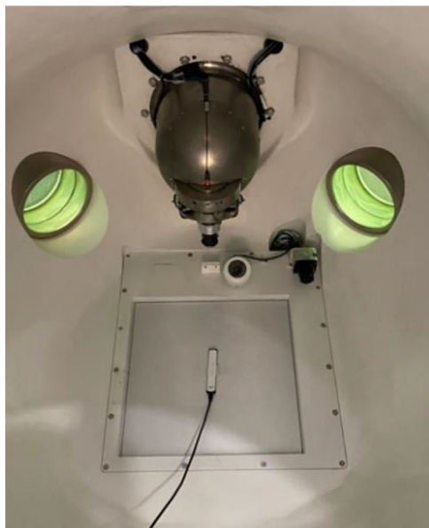
FIGURE 18 X-ray detector setup for kV beam quality/energy measurement. kV, kilovoltage.
