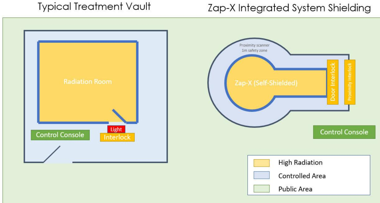
**Figure 27 - A comparison of a traditional Linac installation and the ZAP-X system**
