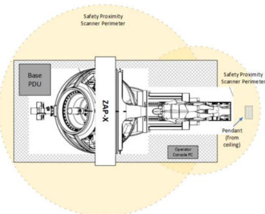
Figure 7 - Floor covering visually defining laser scanner boundary
