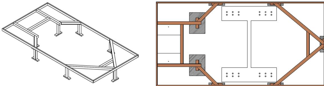
Figure 11 - Pit Floor Frame Construction design
