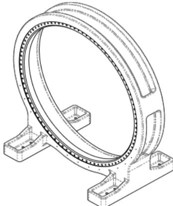
Figure 13 - Module #2 Base Ring
