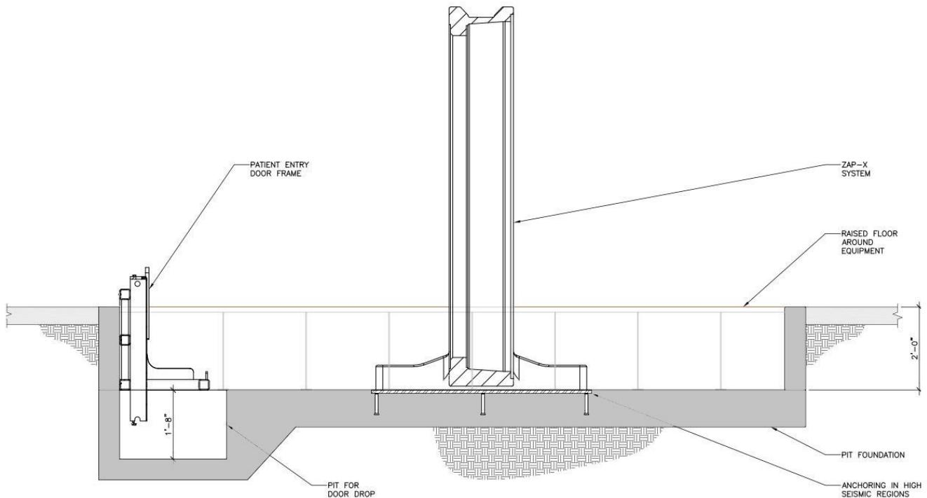
Figure 10 - Cross section view of pit construction
