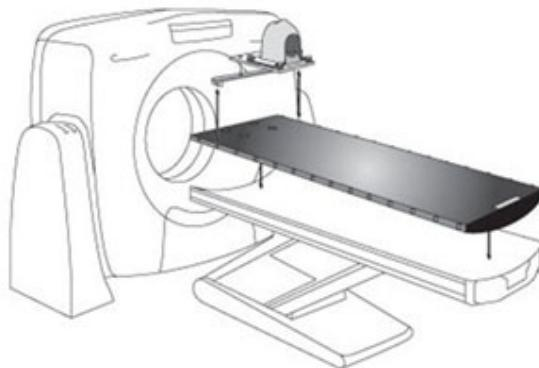
**Figure 24 - Example of CT system with concave couchtop design/flat CT overlay adapter**
