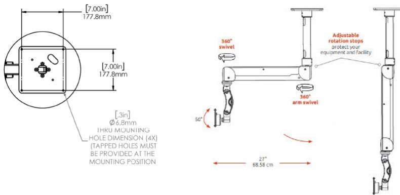
Figure 5 - Example of ceiling mount pendant arm
