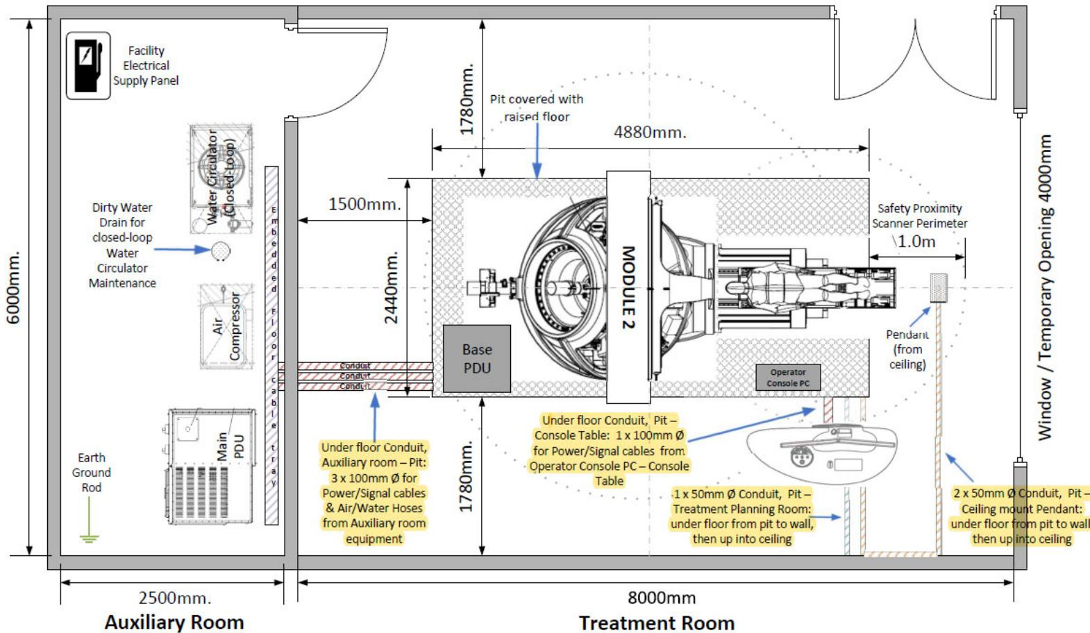
Figure 20 - Typical Room Layout showing conduit locations/paths
