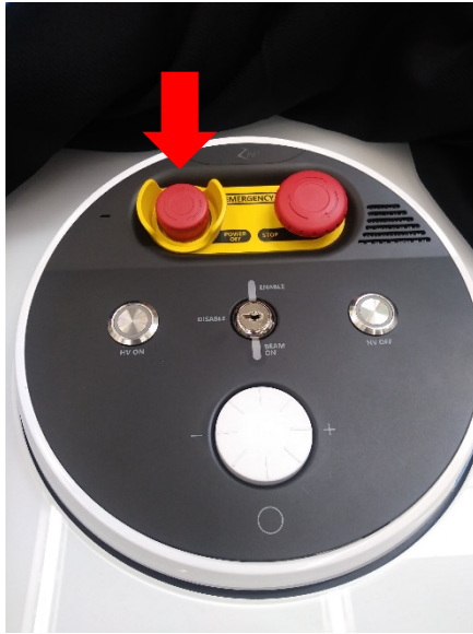
Emergency Power Off Button at the Console
