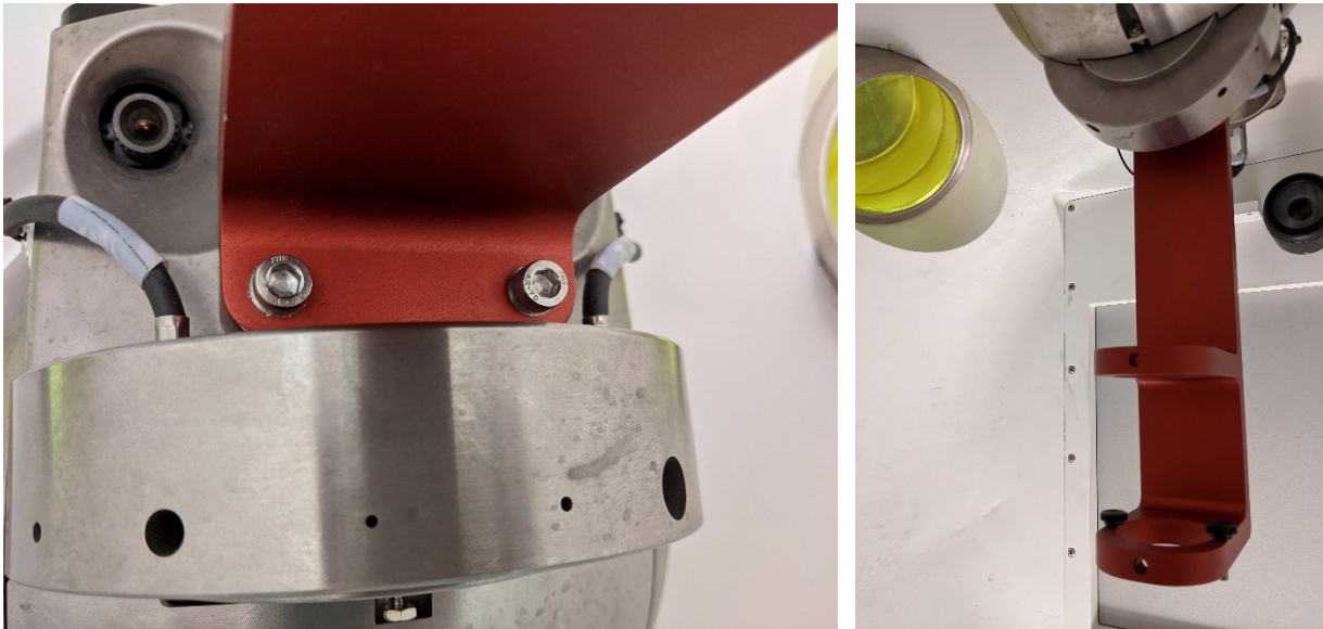
Figure 3-16 Photos of the Zap-X collimator and collimator housing with the F-Bracket installed.
