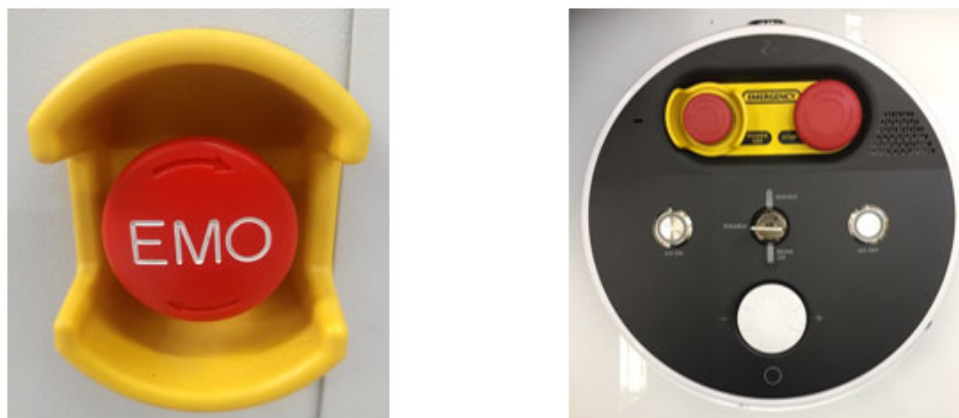
Figure 2.2.1. The EPO button on the PDU (left) and on the operator console (right). Note that the button on the PDU is labeled “EMO” (“Emergency Motion Off”).
