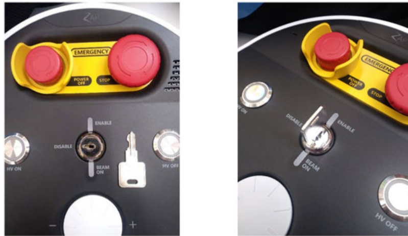
Figure 2.3.1: The HV Enable key
